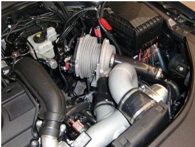
Pic 3 LC Super Hybrid features an electric supercharger developed by CPT. This particular application of its 12-48V switched reluctance motor-generator technology has since been acquired by tier 1 manufacturer Valeo for high volume implementation of the technology.
