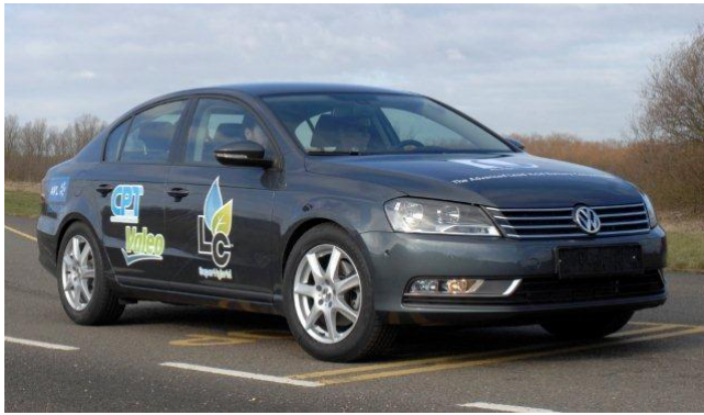
Pic 2 LC Super Hybrid technology demonstrator is based on a VW Passat 1.4-litre TSI model
