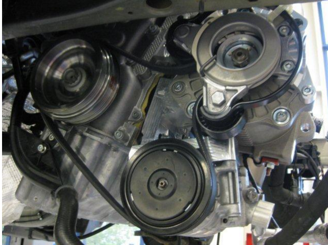
Pic 4 LC Super Hybrid features CPT SpeedStart advanced next generation stop-start technology (top right) and Mubea belt tensioner
