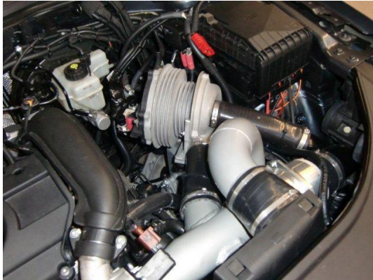
Pic 2 -- 12V and 48V LC Super Hybrid demonstrators feature an electric supercharger developed by CPT and acquired by Valeo for high volume production
