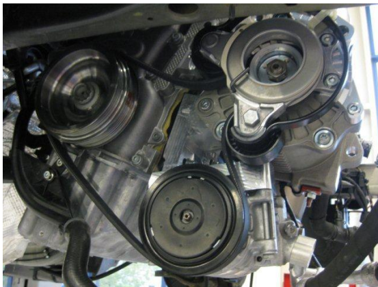
Pic 3 -- 12V and 48V LC Super Hybrid technology demonstrators feature CPT's multiple patent protected SpeedStart motor generator technology (top right) and Mubea belt tensioner
