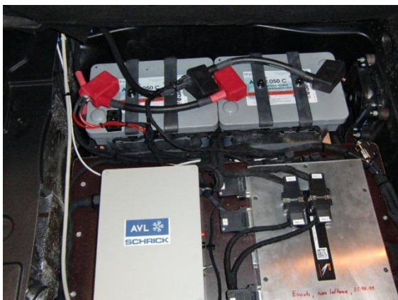
Pic 4 -- 12V and 48V LC Super Hybrid both feature Exide Orbital advanced lead-carbon batteries. Picture shows 12V installation with test equipment, which is eliminated in a production car.
