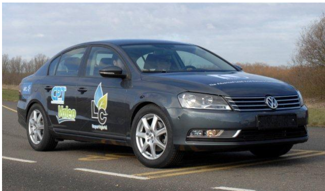
Pic 1 LC Super Hybrid technology demonstrator is based on a VW Passat 1.4-litre TSI model
