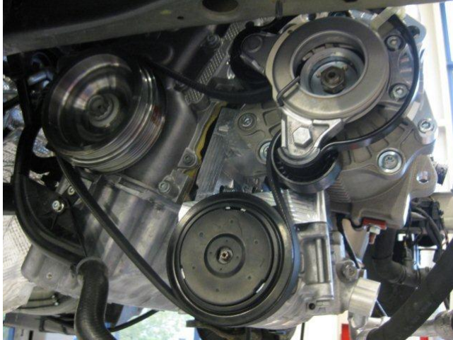
Pic 3 LC Super Hybrid features CPT SpeedStart advanced next generation stop-start technology (top right) and Mubea belt tensioner
