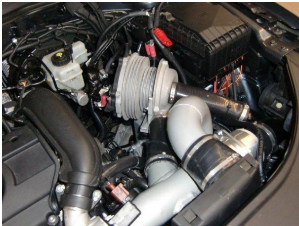
Pic 2 LC Super Hybrid features an electric supercharger developed by CPT. This particular application of its 12-48V switched reluctance motor-generator technology has since been acquired by tier 1 manufacturer Valeo for high volume implementation of the technology
