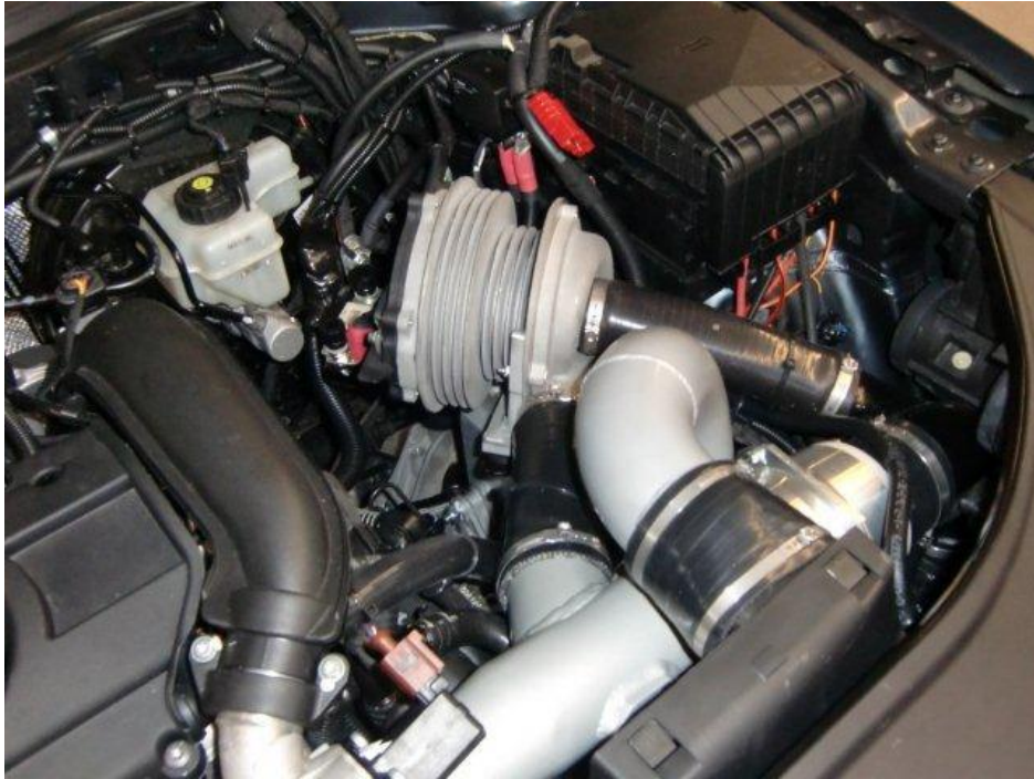
Pic 3 LC Super Hybrids features an electric supercharger developed by CPT. This application of its switched reluctance motor has since been acquired by automotive components manufacturer Valeo for high volume implementation of the technology.
