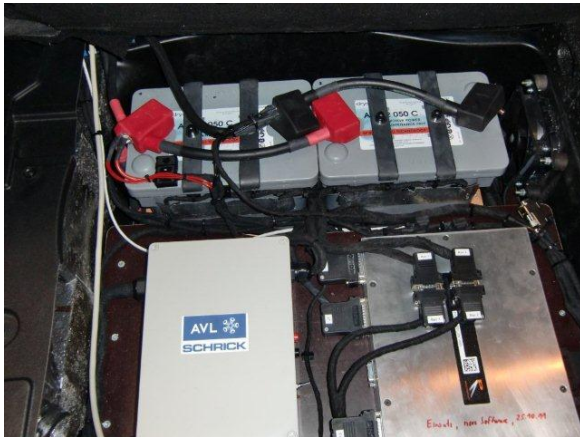
Pic 4 – Low cost LC Super Hybrids both feature Exide Orbital advanced lead-carbon batteries. Pictures show 12V installation (above) and 48V installation (below), with additional AVL test equipment and Provector battery management system in the foreground, which are eliminated in a production car, leaving just a single battery nominally rated at 1kWh.
