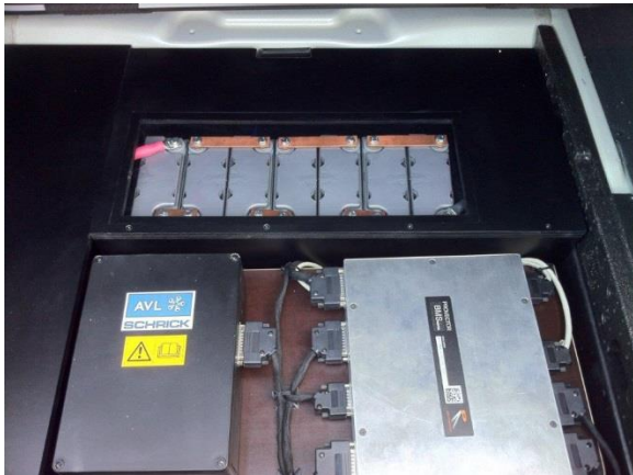
Pic 4 – Low cost LC Super Hybrids both feature Exide Orbital advanced lead-carbon batteries. Pictures show 12V installation (above) and 48V installation (below), with additional AVL test equipment and Provector battery management system in the foreground, which are eliminated in a production car, leaving just a single battery nominally rated at 1kWh.
