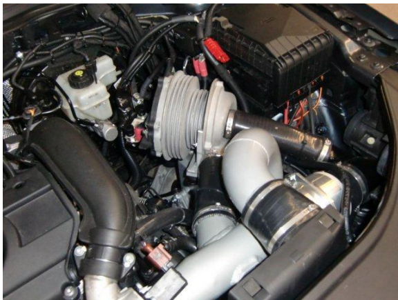
Pic 2 – Low cost 12V and 48V LC Super Hybrid demonstrators feature an electric supercharger developed by CPT and acquired by Valeo in 2011 for high volume production
