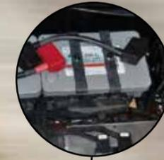
The lead-acid battery has a carbon loaded anode for performance and low cost.
