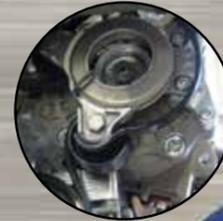
The Mubéa belt tensioner is optimised to minimize friction and guarantee the tension needed for high power transmission.
